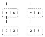
Here each element in the top level list points to one generalized name-value pair, where the name itself is a structure (here a pair of two numbers). REDUCE uses association lists for many different purposes; e.g. if an expression is simplified, the expression and its simplified variant are stored in an association list such that for a second access to the same expression its simplified form is immediately accessible.
